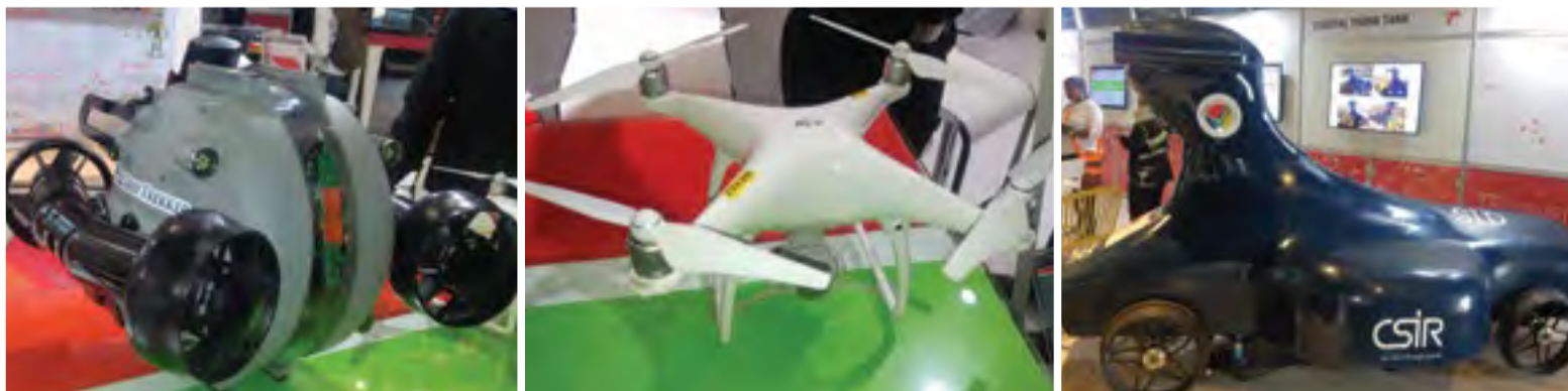
Above: This underwater drone, called Deep Trekker, can go up to 250 m underwater. It was used by Transnet to try and detect three containers underwater that went missing during the recent Durban Storm, which damaged the Port of Durban. Middle: Two types of aerial drones are used by Transnet to track tugs and dredgers and other port resources. It is also very successful to use the drones to inspect infrastructure and the seabed conditions, as well as gathering information on port traffic. Above right: The Special Inspection Device (SID) is the first "drone-type device" built by the Council for Scientific and Industrial Research (CSIR) for Transnet. SID is a fully autonomous inspection device used to detect obstacles, livestock or humans, or defects on the track in front of trains. It is also able to detect cable theft.
